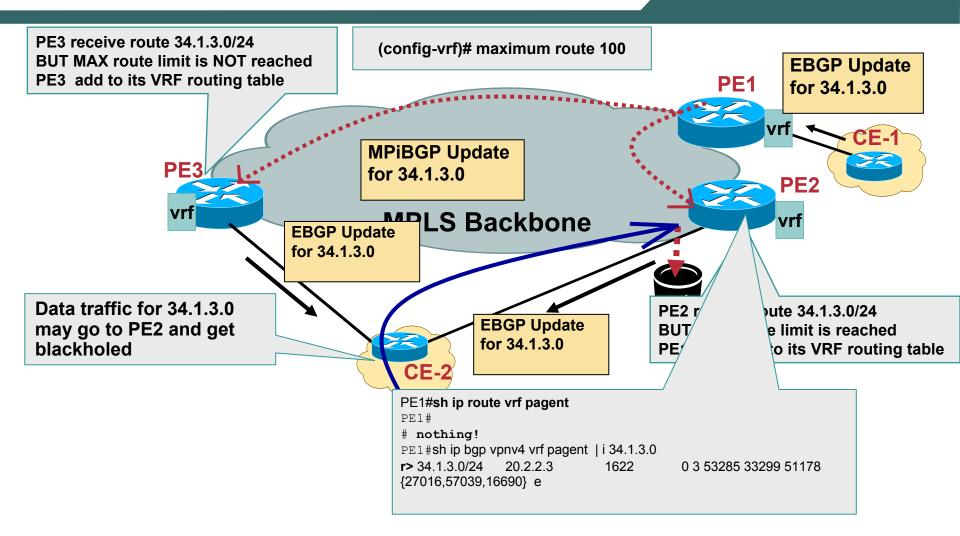
Enable suppress-inactive feature on PE2 to disable advertisements of BGP routes that don't make it to the routing table
