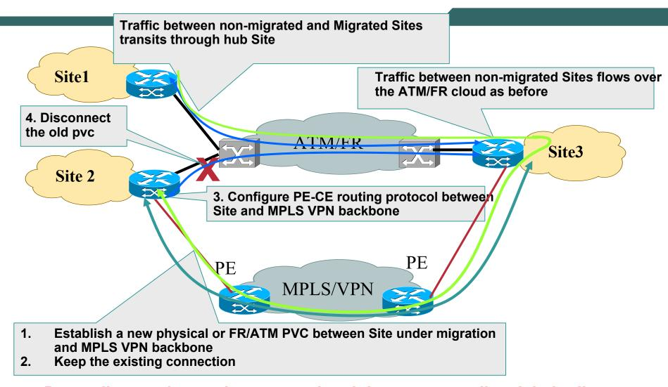
Depending on the routing protocol and the corresponding Admin distance and metrics, traffic will start flowing over MPLS VPN backbone
