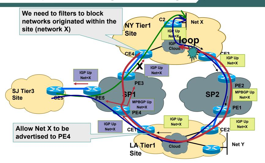
CE4 can possibly choose PE3 as the best path for Net X which can result in suboptimal routing and possible routing loops
