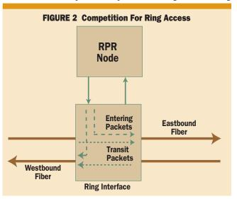
With Cisco's SRP, transit packets take precedence over entering packets, so there's no packet loss on the ring itself. "This is different from how Ethernet switches work," Baher pointed out. Ordinary Ethernet switches, which lack a cut-through path for transit traffic, exhibit varying packet loss throughout the network as traffic congests at each node. If the 802.17 working group decides against transit cut-through, then RPR will lose a potential advantage over ordinary Ethernet switching.
