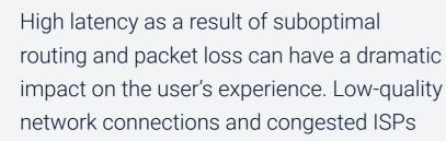
ISP networks increase packet loss in the last mile. Inefficient routing over the long haul (i.e the middle mile) increases latency. Latency can either be tolerated (i.e when using the public Internet) or improved (with SLA-backed and redundant connectivity).
