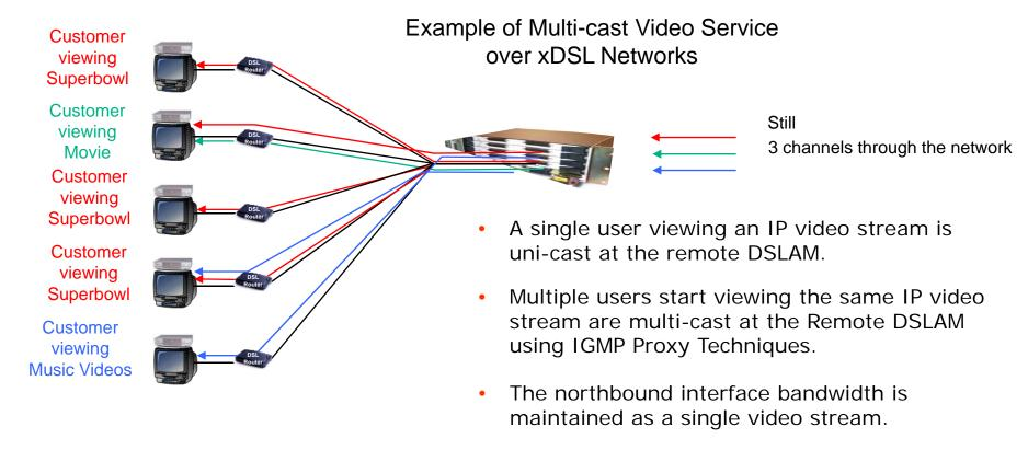
The southbound interface bandwidth is determined upon the DSL service provided, i.e. ADSL2+/VDSL.
