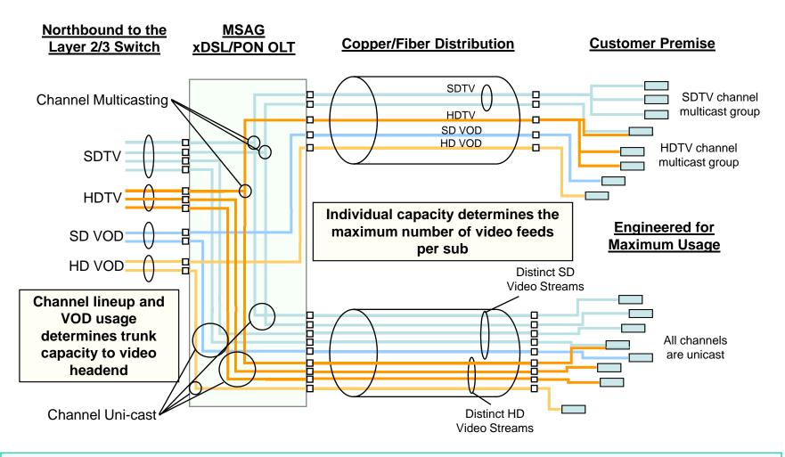
Capacity must meet maximum usage without video blocking for any given take rate.
