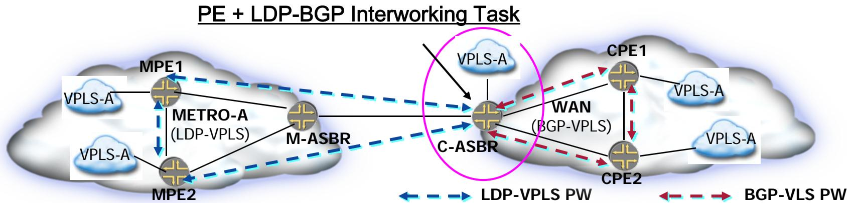
C-ASBR has three mesh groups: one for BGP in the WAN; one for Metro-A; and finally, one for its attached CE(s)
