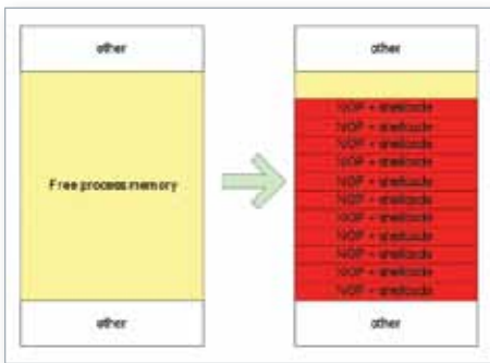
Figure 4. Browser memory sprayed with NOP slides and shellcode.
