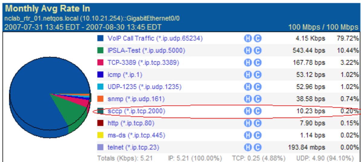
Figure 2-11 – Call setup protocol (SCCP) bandwidth usage on a particular interface
