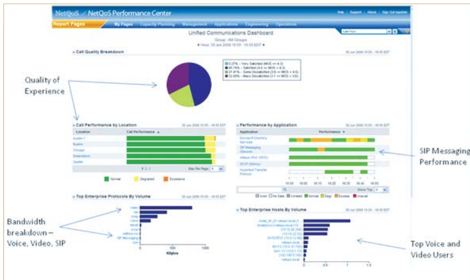
FIGURE 4-6 - A Unified Communications dashboard provides comprehensive view of UC performance
