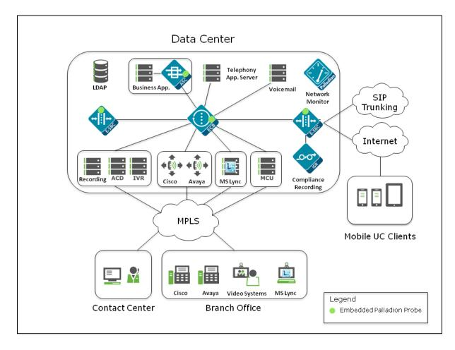
In this large-enterprise vision, the critical elements that run the communication system reside in the enterprise datacenter, which hosts the legacy IP-PBX ("Cisco" and "Avaya" in the schematic) as well as communications applications such as IVR and conference bridging. Also residing in the datacenter is the aforementioned Enterprise Communications Broker, labeled "ECB" on this schematic.
