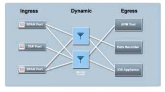
filter is complex and not obvious unless you are well versed in set theory. The port-independent filter is the ideal place to perform the bulk of the filtering as it is possible to understand exactly what is happening by looking at this single filter definition. When considering a network monitoring switch it is important to understand its filtering capabilities. Please refer to the diagram above for an example of three stage filtering.
