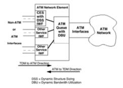
DBCES can operate in either PVC or SVC ATM network configurations. The active time slots are transmitted using the standardised CES service.
