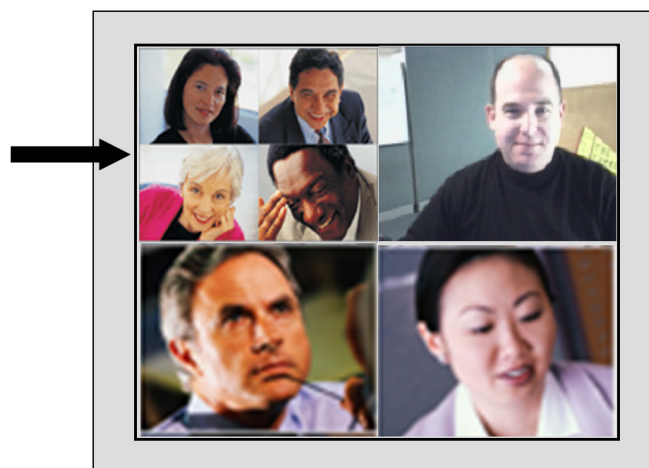
Figure 9. Picture-in-Picture Effect From Some Cascading MCUs
