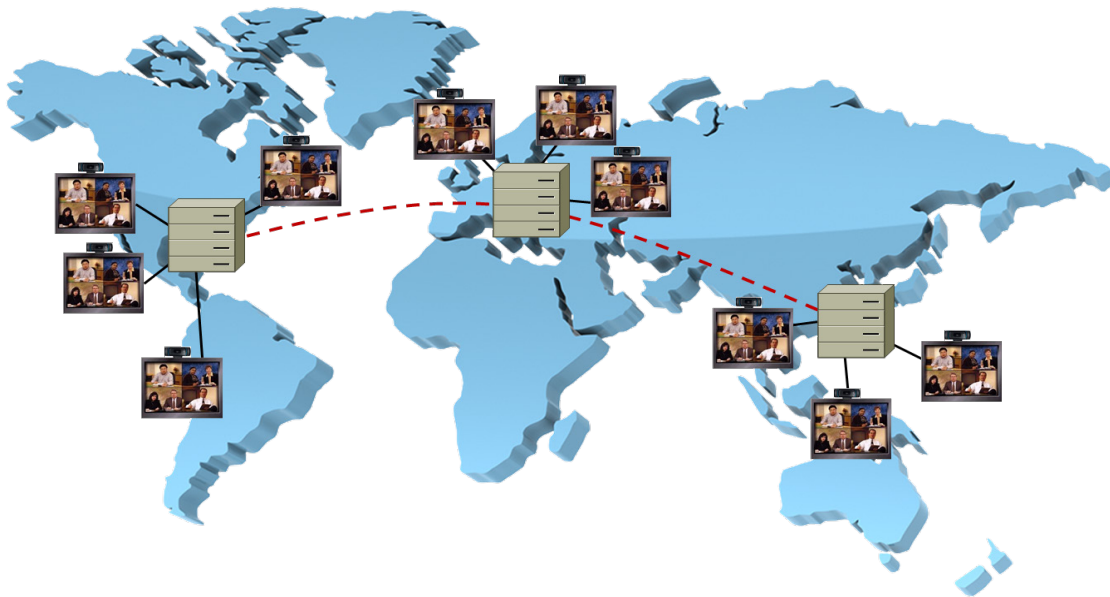
Figure 8. Cascading Video MCUs or Video Routers
