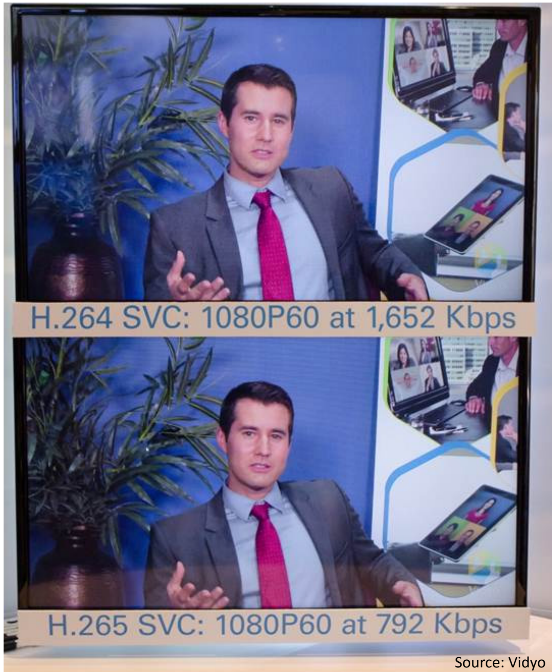
Figure 5. Comparing H.265 SVC Image Quality and Bandwidth with H.264 SVC Video.
