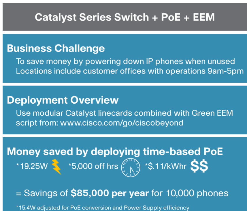
Figure 5. Time-based PoE Using Embedded Event Manager (EEM)
