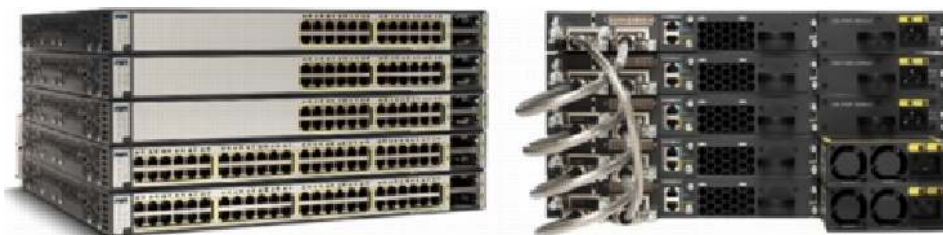
Figure 11. Cisco Catalyst 3750E Stack
