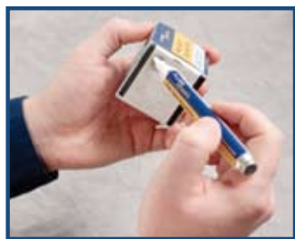
Figure 15 – “Wet to dry” cleaning methodology. Apply a small spot of solvent to the starting edge of a wipe. Holding the end-face connector perpendicularly, swipe the end-face from the wet spot to the dry zone.
