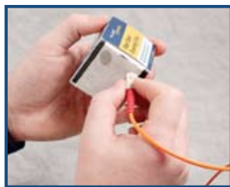
Figure 15 – “Wet to dry” cleaning methodology. Apply a small spot of solvent to the starting edge of a wipe. Holding the end-face connector perpendicularly, swipe the end-face from the wet spot to the dry zone.
