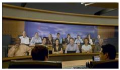
The Polycom RPX 400 Series has an enourmous 4 foot x 16 foot video wall that takes up almost the entire peripheral vision of the eye, the camera is hidden at eye-level behind the screen, the participants are perfectly positioned, and the architectural elements of the room are mirrored to produce a superb sense of immersion.
