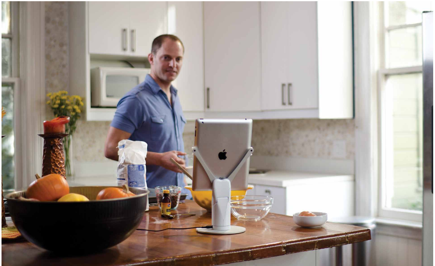
The Revolve Robotics Kubi holds a video-enabled tablet or smartphone that can be controlled by a remote participant for a more fluid and natural video call.
