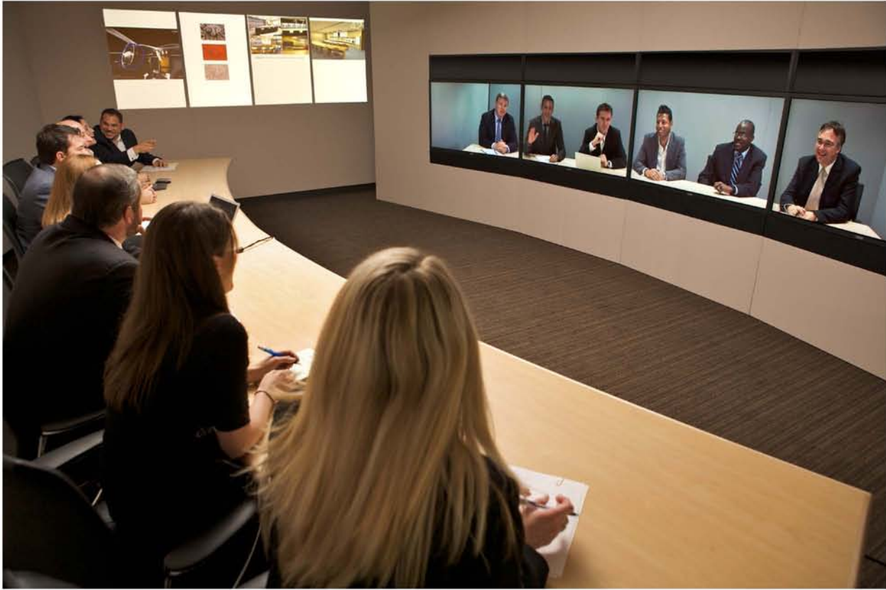
Teliris VirtuaLive uses SVC to traverse bumpy networks. It's available as either an engineered environment that unifies the look and feel of each location or as a modular, stand-alone system installs with little make-ready
