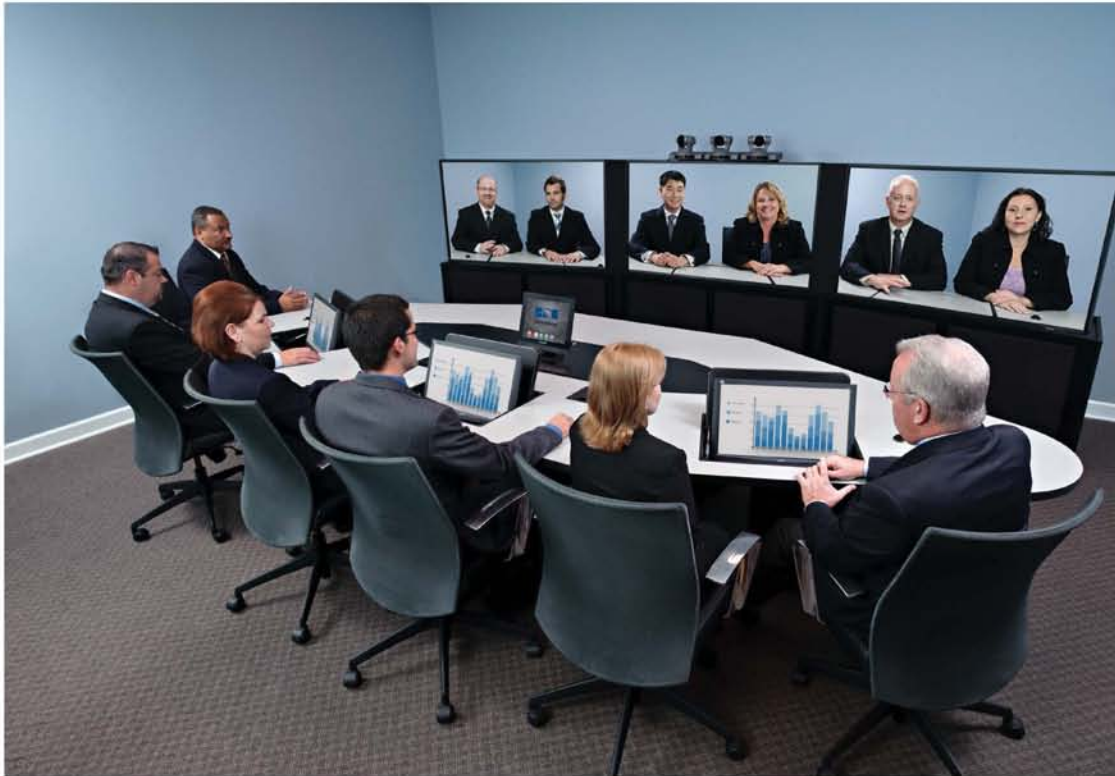
The AVI-SPL Camèlèon is a modular group telepresence system that can be deployed with Polycom, LifeSize, or Cisco C 40 codecs. The system can be installed in one day and the control system can be configured to control everything from room lighting to collaborative peripherals.
