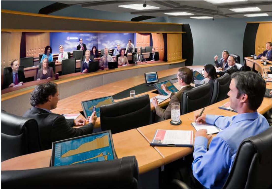
The Polycom RPX 400 Series can seat up to 28 participants and make each of them visible on-screen. Its telepresence multipoint ability can connect five sites and display seven participants on the screen from each of four locations—a total capacity of 140 participants.
