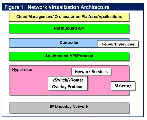
The most common approach is to perform the encapsulation at the hypervisor vSwitch, which acts as the network virtualization edge (NVE). As a result, overlay NV solutions can generally be implemented over existing networks without requiring any changes.
